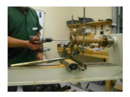
Before hollowing, Don always drills to the required depth. His preferred method is to use a drill rather than the lathe. He uses a masonry bit sharpened like high speed bit. This works out much cheaper than buying an extra long series bit. The tungsten carbide masonry drill costs around \$15 and he has it sharpened by an engineering workshop for about \$10.
