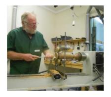
His preferred tool of late is the Easy Hollower by Easy Tools. Once again, the cut is made at centre with the tool horizontal to the bed. In all cases a firm grip is used with the tool. As can be seen above right, the tool is held under the forearm with the elbow tucked into and braced by the waist. It is essential that the tool is supported directly behind the cutting edge on the tool rest.
