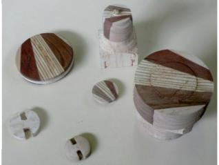
President Dianna is challenging members to make buttons, toggles and pins which are featuring in the fashion world. David Scott produced some samples of a method of producing buttons by gluing together different coloured timbers and making a backing piece with a hole drilled through it which can be glued on the back so that they can be sewn on to material.
