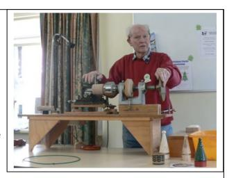
The small electric motor Cliff uses to drive the cutters comes from a sewing machine and connects with a narrow plastic type belt. This belt can be cut to the length needed and joined by gently heating the ends before holding together – remembering that heated plastic can hold its heat and stick to fingers.
