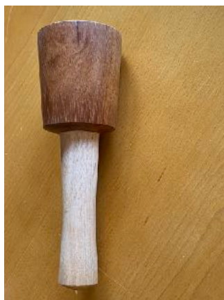
Roger Annells, a wooden mallet with a Merbau head and a Tasmanian Oak handle. Finish Danish Oil.
