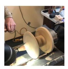
and the other piece of plywood has a hole which fits over the turning. When the nuts on the allthread rods are tightened, the turning is held securely to enable turning to be done. This was also turned to a point, a template used to ensure the profile matched the other end.
