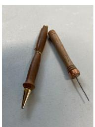
Di Bermingham altered a slimline pen into a needle threader, but before she could slip the new fine wire into the old cartridge she needed to make a tool to knock the ball out of the cartridge
