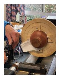
If the fit of the bowl is a tiny bit loose use a piece of paper towel in between the bowl and the blocks to give a tighter fit.
