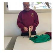
Alan Thompson showed a jig he made to use instead of Cole Jaws. The jig was made from plywood and is adjustable to suite different size bowls
